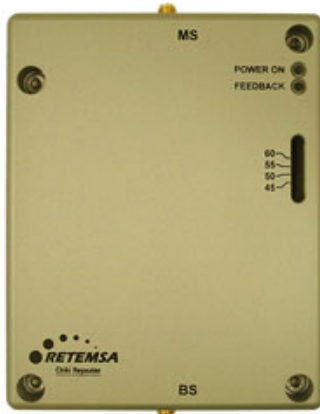
MODEL CHIKI-19xxi GSM 1900 MHz / 13 dBm
